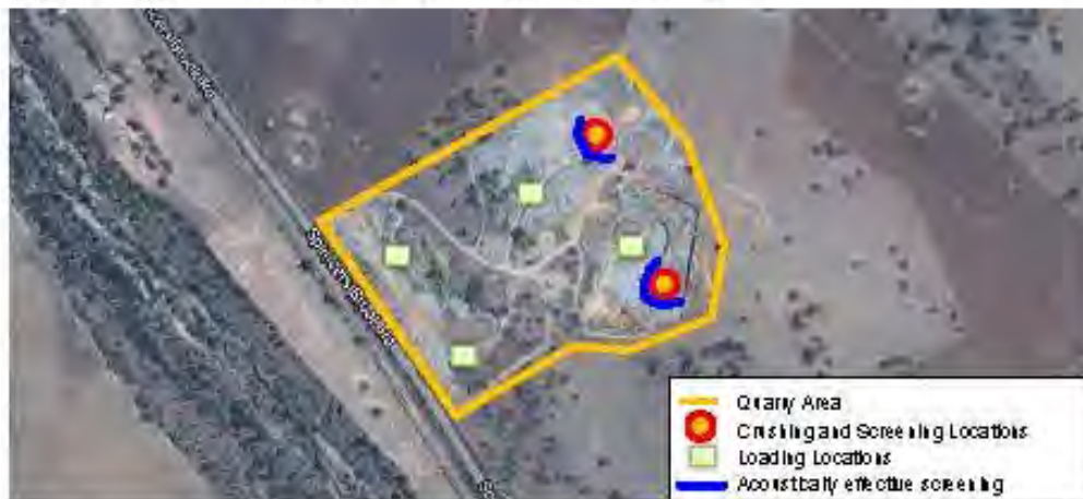
Figure 4 Approximate Location of Acoustically Effective Screening
