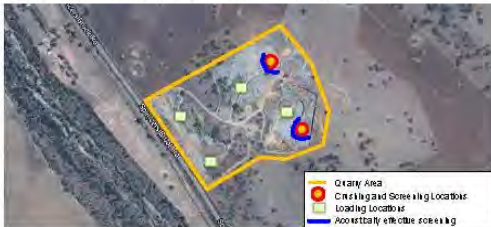
Figure 4 Approximate Location of Acoustically Effective Screening
