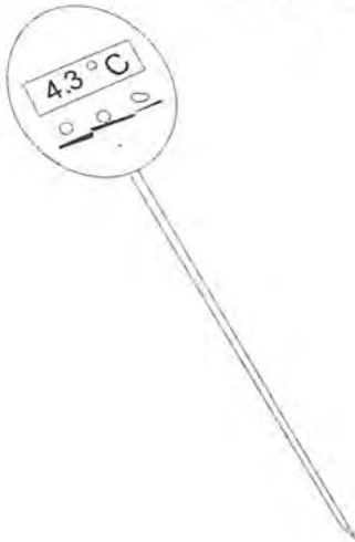
Figure 10: example of temperature measuring device accurate to +/- 1°C
