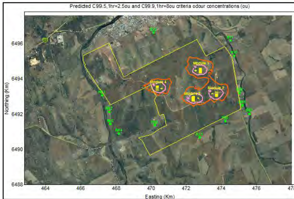
Figure 14 Predicted C99.5,1hr=2.5ou and C99.9,1hr=8ou criteria odour concentrations (ou)
