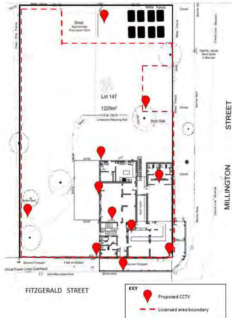
Figure 13 Proposed CCTV installation
